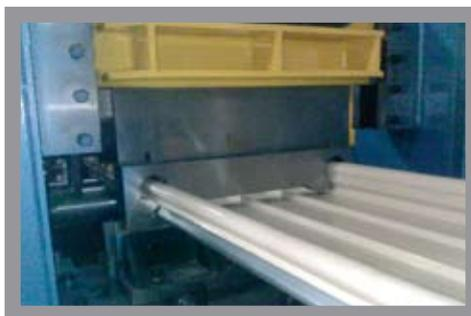
Roll formed Pre-Painted Steel Roofing manufactured by Classic in Western Australia
